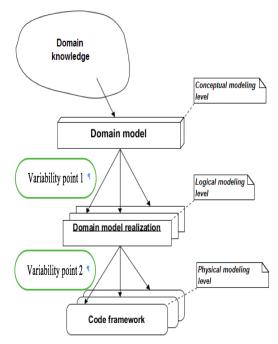
Figure 3: 3-level scheme in DDD approach.
