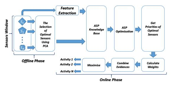
Figure 16: Reasoning system structure for activity recognition
