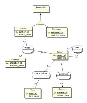
*Figure 4: Example of conceptual model (Akoka et al. 2017)*
