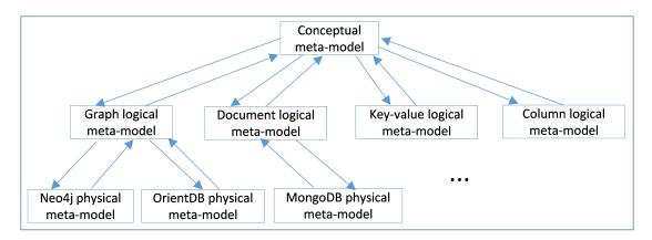
Figure 3: Recommended paths for NoSQL database roundtrip engineering
