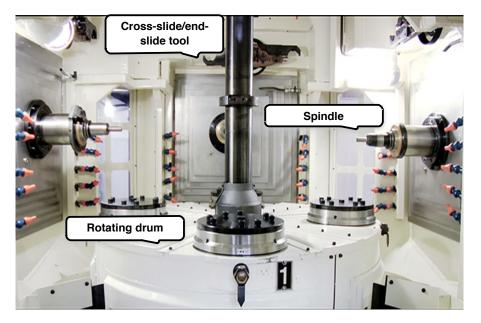
Figure 1: Multi-spindle machine considered for the running example.
