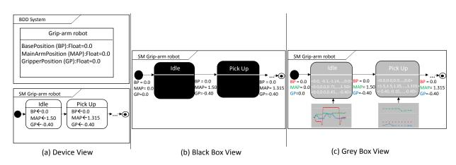
Figure 1: Different model-based views on a grip-arm robot.
