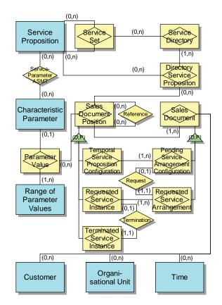
Figure 6: Data structure for service arrangement configuration [eERM]
